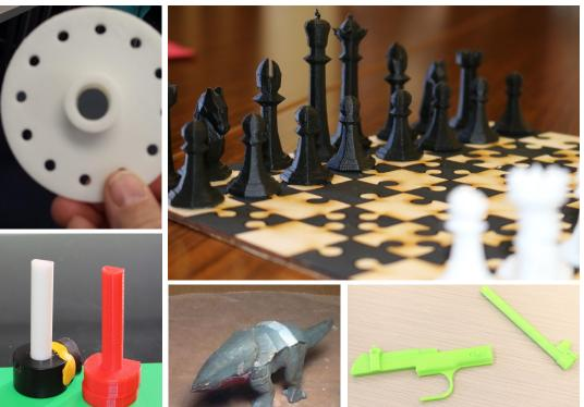
3D printed projects. *From left to right:* Plain, white ABS hedgehogs, with acrylic painted smaller model; White ABS magnetic rotating disk for a camera; Black and white ABS chess pieces with laser cut and painted jigsaw chessboard; Laser focus tool and red ABS copy; Red ABS dinosaur painted silver; Custom-designed, green PLA blaster prop for Star Wars-themed costume.
