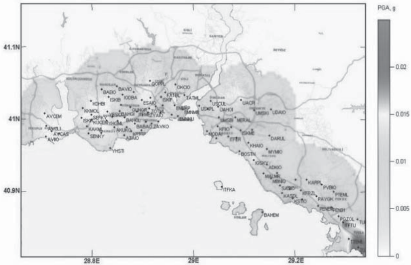
Figure 10. Distribution of peak ground acceleration (PGA) in Istanbul caused by the 06.05.2004 (Md=4.5) earthquake in the Marmara Sea.
