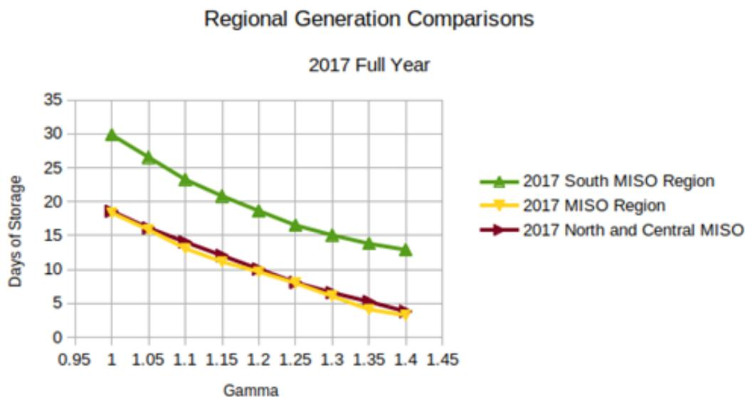
Figure 5: A plot depicting the regional breakdown of the MISO region. These days of storage correlate to a zero deficit energy. Generation based on data from NREL and MISO.
