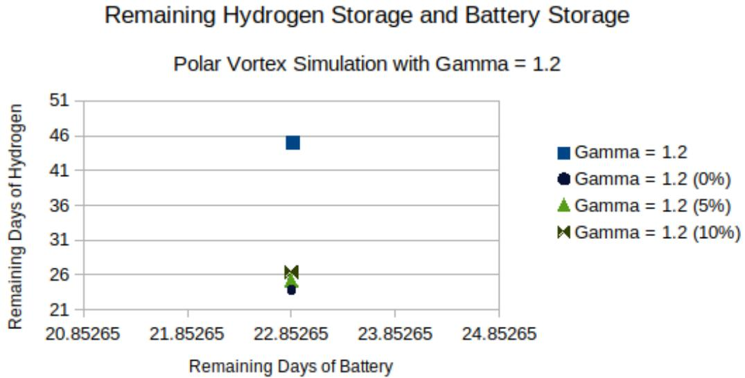
Figure 8: A plot showing the remaining days of hydrogen and the remaining days of battery storage after the 2-week polar vortex event given a gamma of 1.2. The “strongest” polar vortex (i.e., 0% generation) guarantees 26.5 days of hydrogen after the simulation’s end.
