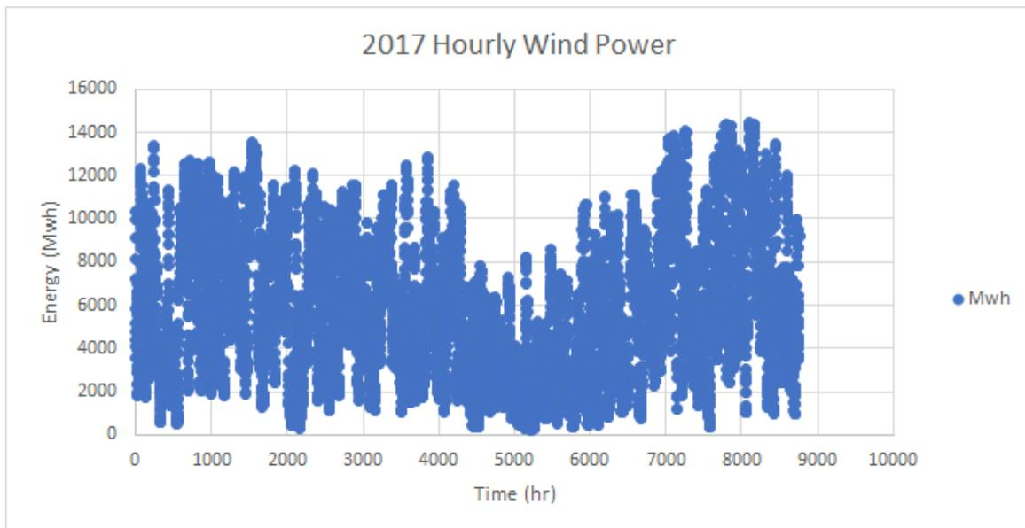
Figure 12: A plot of the hourly wind power generation for 2017. From the MISO database.
