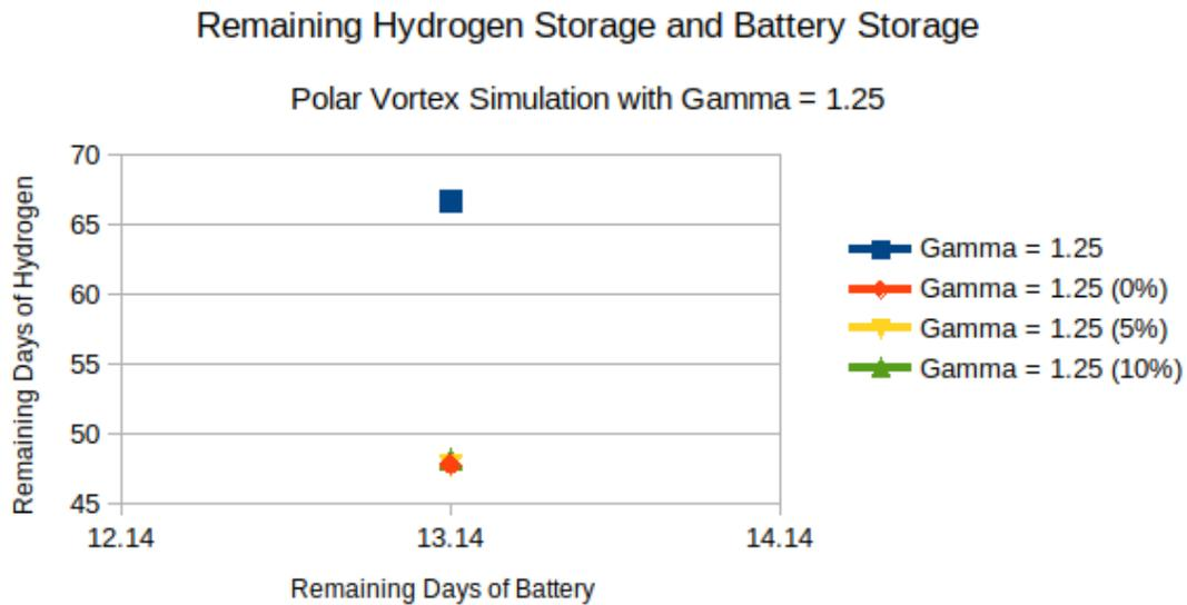
Figure 9: A plot showing the remaining days of hydrogen and the remaining days of battery storage after the 2-week polar vortex event given a gamma of 1.25. The “strongest” polar vortex (i.e., 0% generation) guarantees a minimum hydrogen storage of 48 days.
