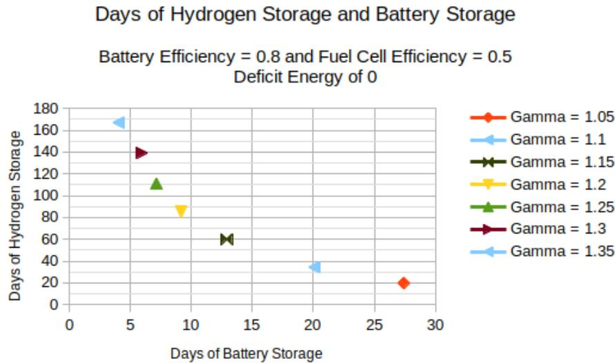
Figure 6: A plot depicting the days of available hydrogen storage against days of available battery storage. Greater gamma corresponds to more hydrogen storage and less battery storage.
