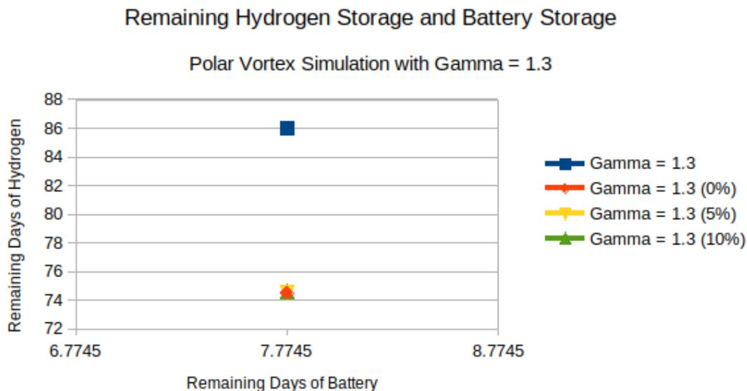
Figure 10 A plot showing the remaining days of hydrogen and the remaining days of battery storage after the 2-week polar vortex event given a gamma of 1.3. The “strongest” polar vortex (i.e., 0% generation) guarantees a minimum hydrogen storage of 74.5 days.
