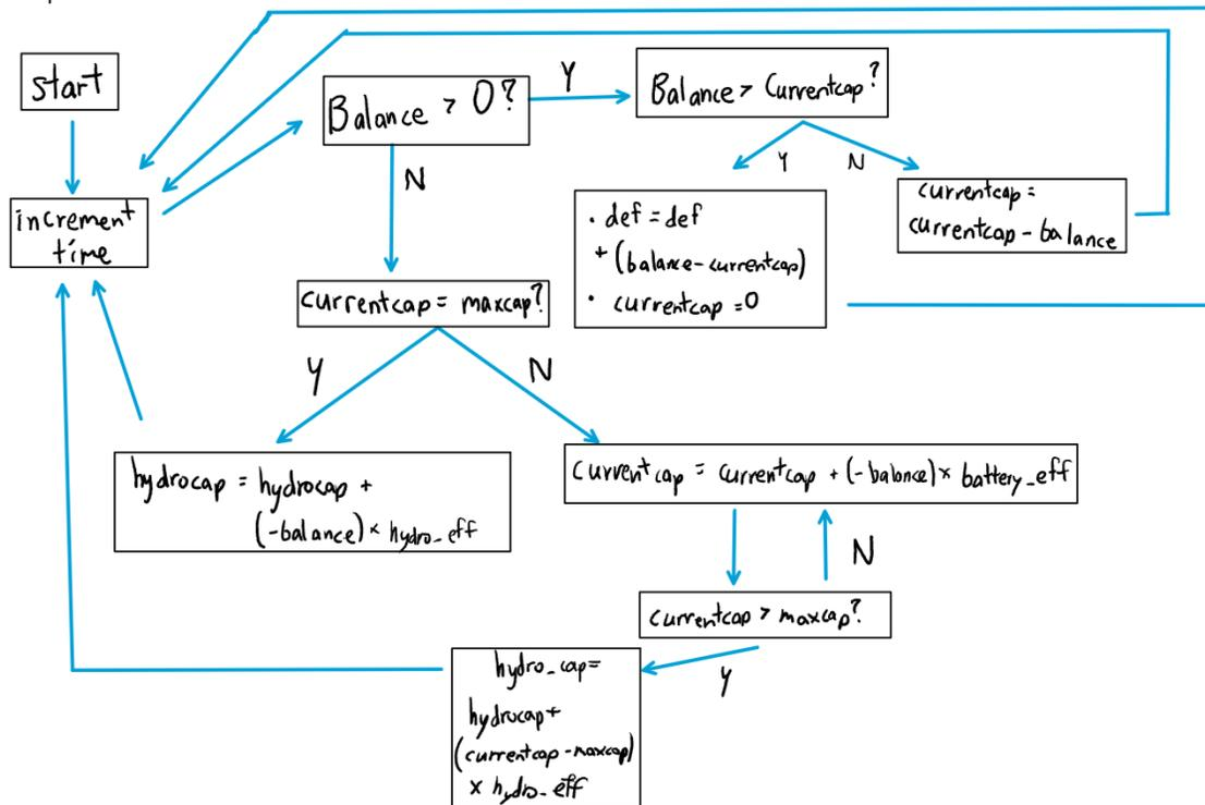
Figure 2: Flowchart of the foundational code used to track battery and hydrogen storage for the three-year period. The code is centered on calculating the balance at each time step and comparing it to the current battery capacity. Spill goes to hydrogen.
