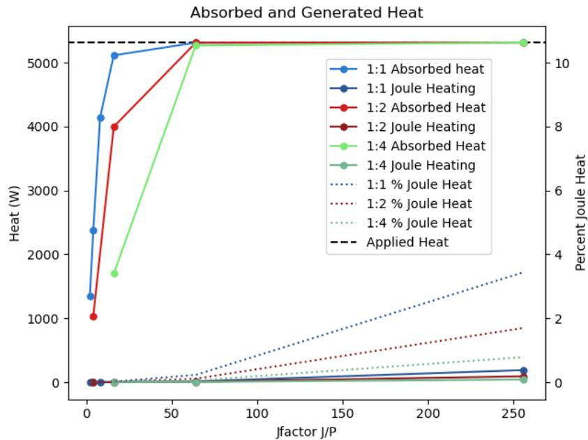
FIG. 9: Absorbed heat and Joule heat as a function of increasing current. All aspect ratios absorb nearly all the incident heat at large enough currents. However, the largest aspect ratio channels generate more joule heat and thus are less efficient than the smaller channels (as seen in the dotted lines).
