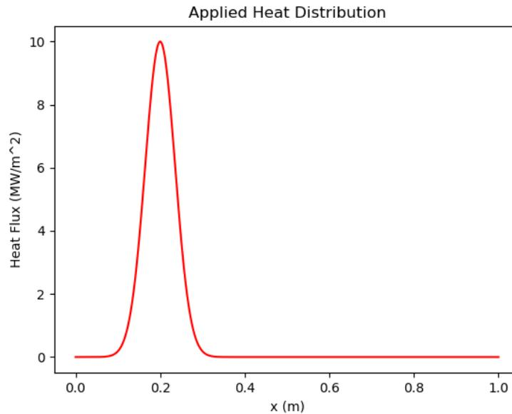
FIG. 3: A gaussian heat distribution applied to the porous surface. At low channel temperatures, all applied power is. At higher temperatures, the absorbed power decreases linearly from the value shown in this plot to account for evaporation.
