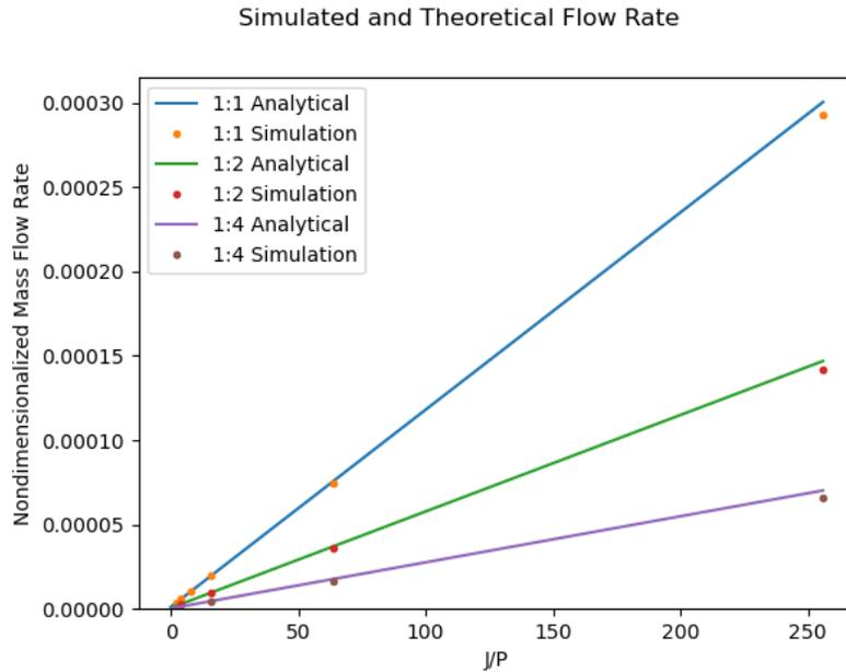
FIG. 7: Comparison between simulated and analytical flow rates as a function of applied current for 3 different aspect ratios. The difference at large currents is due to the conductivity of the electrodes, which is assumed infinite in the analytical solution.
