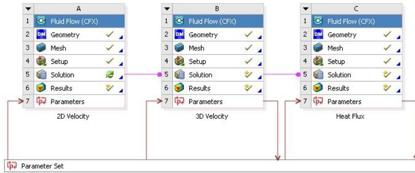
FIG. 5: ANSYS Workbench setup. The 3 blocks calculate a 2D velocity profile, the 3D velocity field, and then heat transfer on the frozen velocity field. All three blocks pass parameters back and forth with the parameter set block, which allows the same setup to evaluate different currents and channel geometries.
