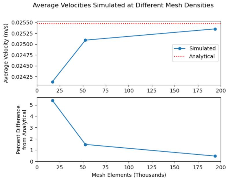
FIG. 4: The upper plot shows the average velocities calculated by ANSYS at several mesh densities. The lower plot shows the percent difference between those velocities and the velocity calculated by Shercliff<sup>3</sup> (Equation 1), which is displayed as the dotted line in the upper plot as well. It seems that as mesh density increases, the simulation is converging towards the analytical solution.
