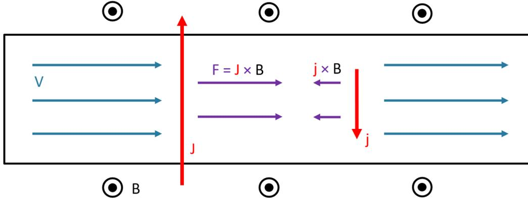
FIG. 1: A magnetic field pointing out of the page induced a downward current ( $j$ ) in conductive fluid flowing to the right. This current creates a drag force opposing the direction of the flow. Passing a larger current ( $J$ ) upwards through the fluid creates a force in the direction of the flow, increasing the velocity.
