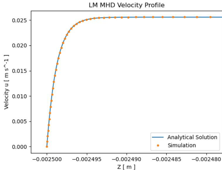
FIG. 6: Comparison between the simulated velocity profile and Hartmann's result (Equation 2) shows good agreement. This is only a small portion of the width of the channel because the boundary layer is thin (approximately  $1/M$  of the width of the channel<sup>3</sup>) and the flow is dominated by the uniform core flow
