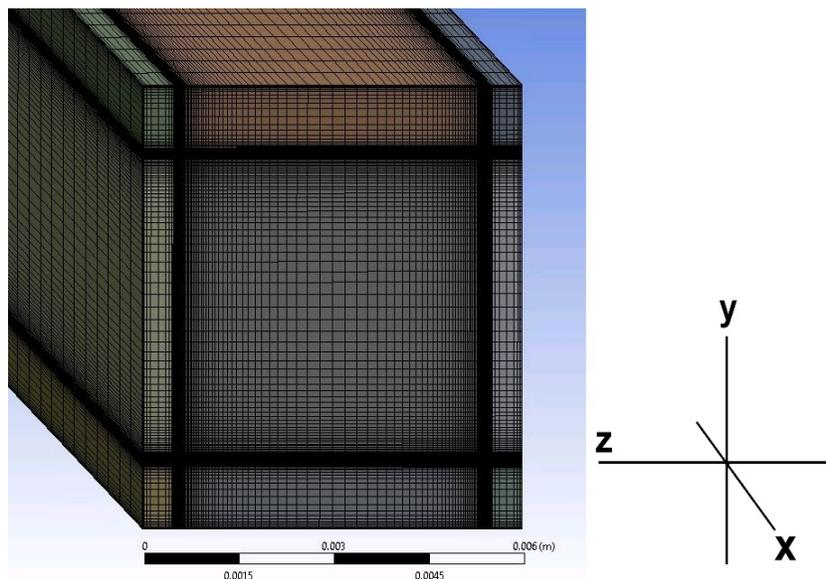
FIG. 2: The ANSYS model with the mesh displayed. The mesh is coarse in the walls and at the middle of the liquid channel where high resolution is not required to achieve a good solution. The mesh density is much higher near the interfaces between the liquid domain and walls where boundary layers are expected and need to be resolved.
