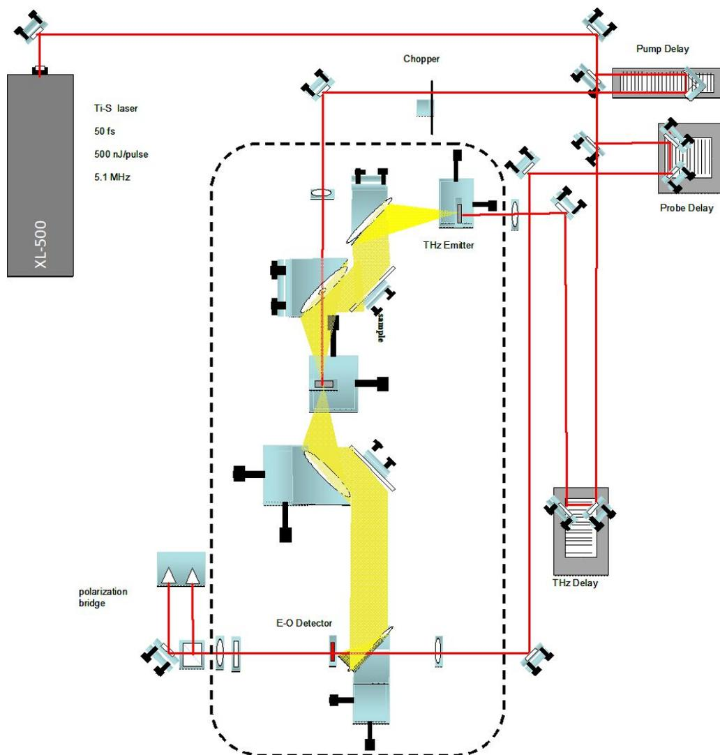
Figure 1. A diagram of the laser system. A yellow beam represents terahertz radiation, a red beam represents 800 nm light. The sample is located at the small grey rectangle in the center of the diagram.
