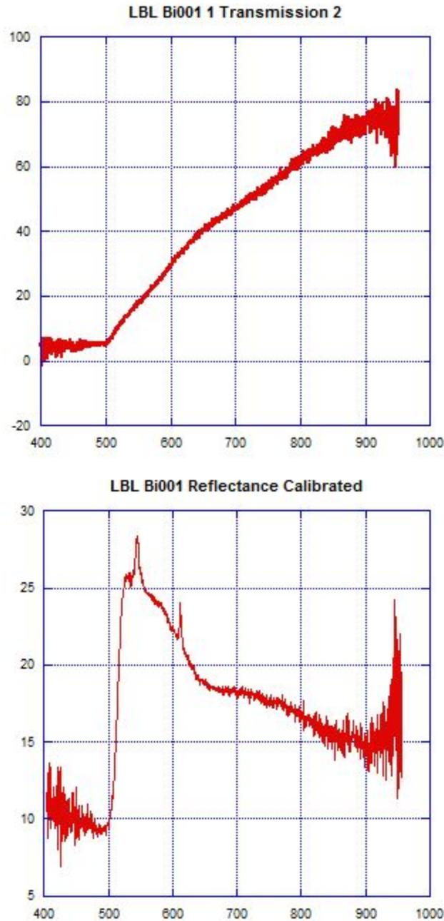
Figure 4. Transmission and reflection graph of a degraded sample. Percent of light transmitted (upper) or reflected (lower) on the y axis, wavelength of incident light on the x axis. Compared to Figure 2, transmission has increased on all wavelengths, the bandgap completely vanished. The reflectance has also shifted to be higher at smaller wavelengths.
