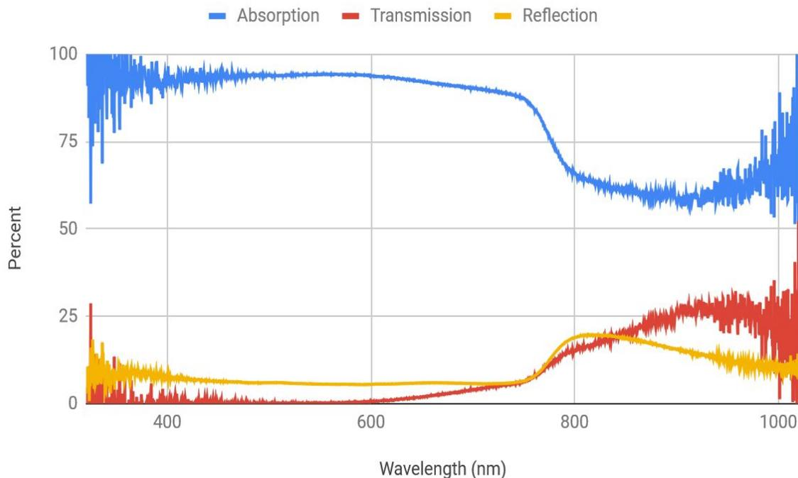
Figure 3. This is the transmission and reflection graph of a sample with 0.50% bismuth. Percent of light transmitted (red), reflected (yellow), or absorbed (blue) on the y axis, wavelength of incident light on the x axis. The value significant to us is the one at 800 nm. Tests at 400 nm were also tried due to the higher level of absorption at that wavelength, but were too damaging to the sample to continue.
