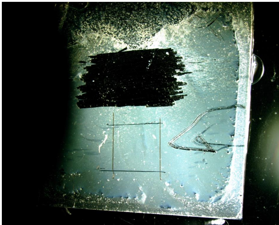
Figure 1: This is an image of one of our samples. It shows how inhomogeneous our sample surfaces were. It also shows one of the electrically isolated squares and reference areas.
