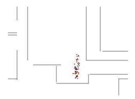
Figure 2: Distributed sample points surrounding robot
