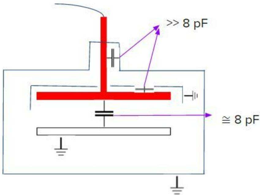
**Figure 2.** Simplified schematic of chamber showing all the possible places for capacitive effects to occur. Red denotes powered. The capacitance produced by interactions with the chamber walls and the electrode shield are much greater than the capacitance produced between the two electrodes.
