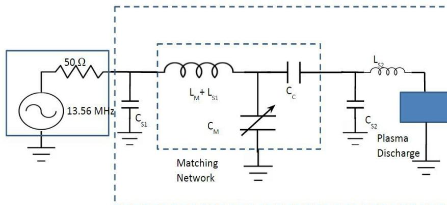
Figure 1. Schematic showing entire circuit design. Small dashed box denotes contents of matching network. Large dashed rectangle represents the components whose total must equal  $50\ \Omega$  in order for no reflected power.
