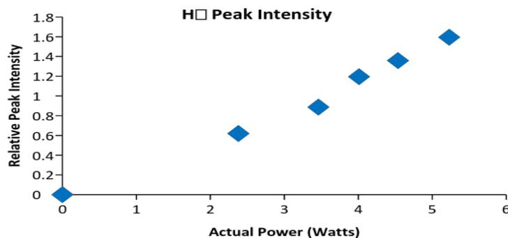
Figure 3. Plots showing  $H_{\alpha}$  (red) and  $H_{\beta}$  (blue) relative peaks area on the y-axis versus actual power delivered to the discharge on the x-axis.
