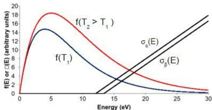
Figure 6. Plot showing cross sections  $\sigma_\alpha$  and  $\sigma_\beta$  intersecting with the Maxwellian average electron energy function  $f(E)$ . The x-axis is energy in electron-volts and the y-axis is the function  $f(E)$ , known in this case as the probability the electrons has the correct amount of energy.
