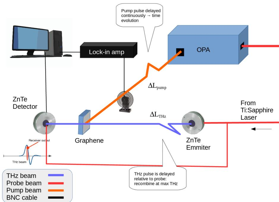
FIGURE 2. A conceptual diagram of the experimental setup. A Ti:Sapphire laser emitting 120fs pulses at  $\lambda = 800\text{nm}$  with a 1KHz repetition rate powered the OPA as well as the THz and probe beams.
