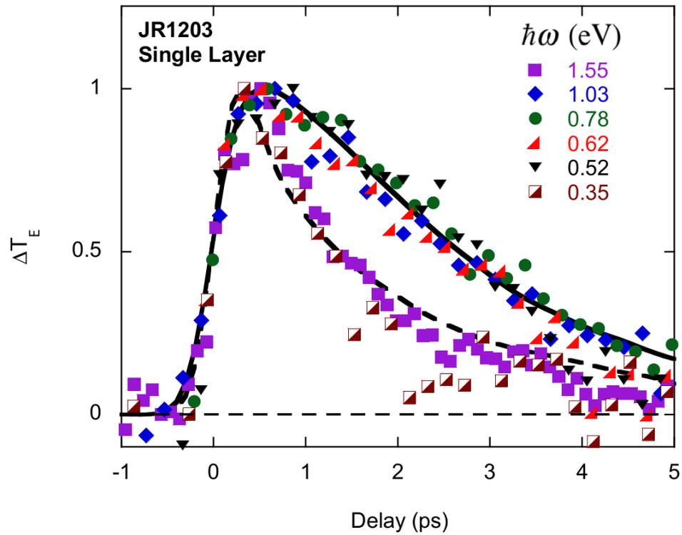
FIGURE 4. Time-resolved change in THz transmission versus delay. Curves are normalized based on long range determination of transmission. Solid lines indicate contours of absorbed pump intensities:  $400 \mu\text{J}/\text{cm}^2$  (solid)  $40 \mu\text{J}/\text{cm}^2$  (dashed). [4]
